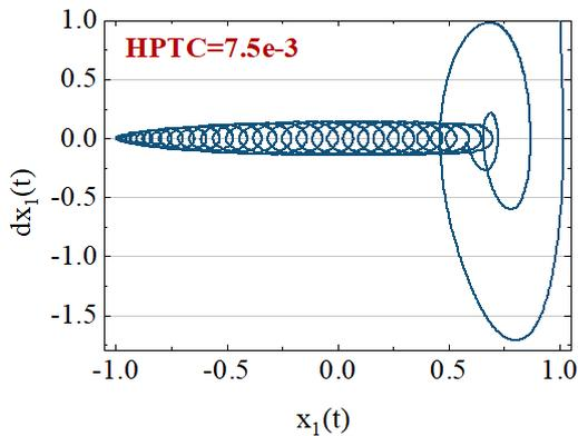
**Fig. 2** Output phase diagram of the Duffing system,  $A = 0.029$ .
