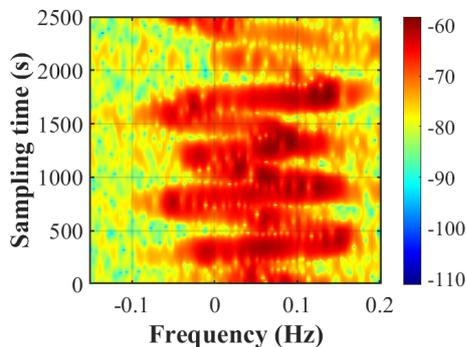
**Fig. 3** The time-frequency distribution of gravity wave features.
