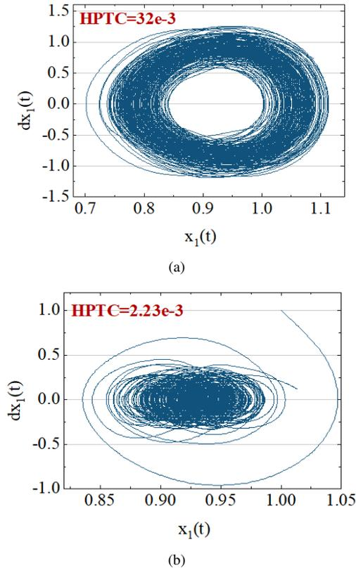
**Fig. 5** The chaos detection results. (a)  $s(t)$  is the time series of gravity wave features with target signal. (b)  $s(t)$  is the time series of gravity wave features without target signal.
