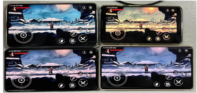
Fig. 13 Four of eight instances are running concurrently on Server II (from left to right, and from top to bottom, the terminals are Huawei Mate 20, Google Pixel 3, Huawei P40 pro and Huawei Mate 40 pro).
