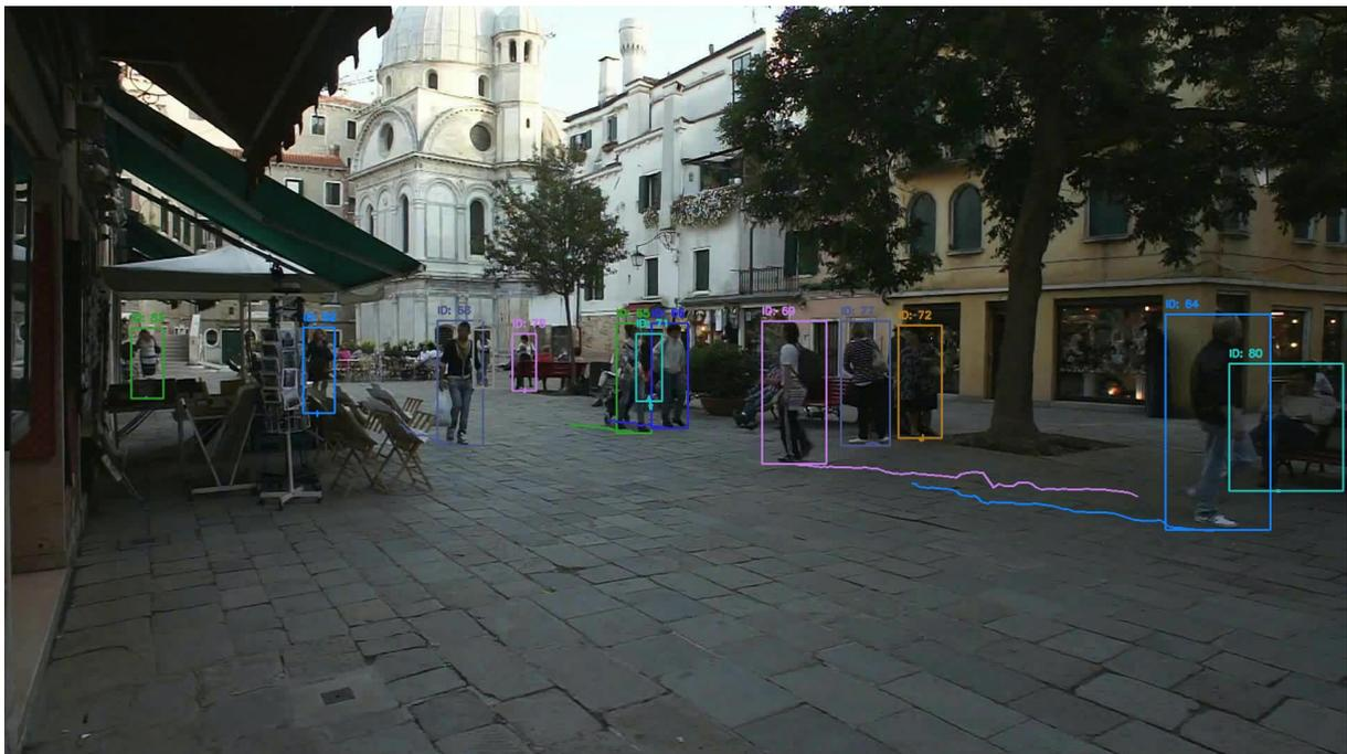
**Fig. 8** Tracking performance of DETrack on object long-distance movements trajectories.
