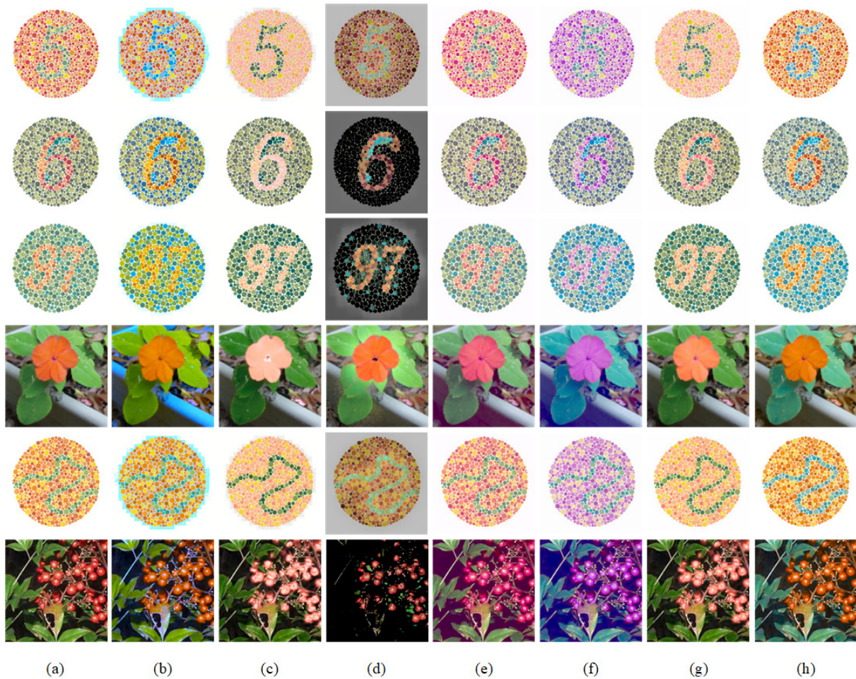
Fig. 10 Recolor images of D-type color perception method: (a) Original, (b) Milic, (c) Takimoto, (d) Tennenholtz, (e) Hassan 2017, (f) Hassan 2019, (g) Meng, and (h) Proposed.
