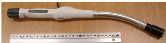
Fig. 12 Measurement device based on J & J circular stapler.
