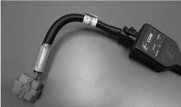
Fig. 2 Example of device for diagnostics in CAN communications. Depicted is a replacement that fits into the OBD-II port.
