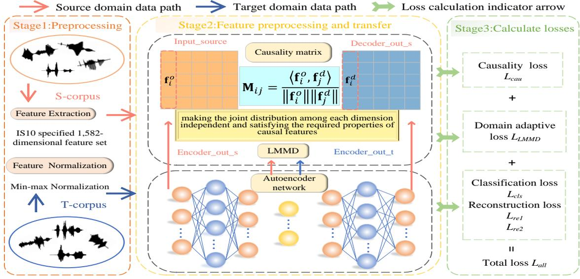
Fig. 1 Cross-corpus speech emotion recognition model framework based on CEIR
