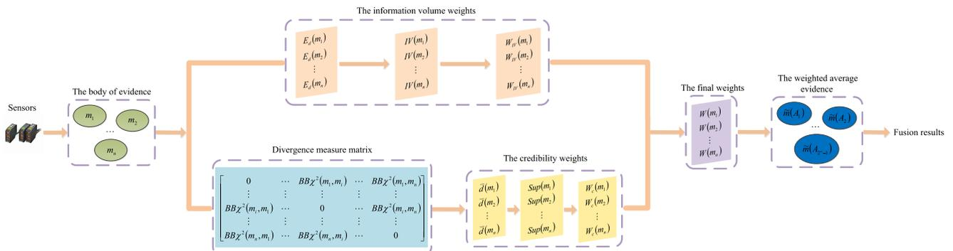
Fig. 4 The flowchart of the proposed multi-source information fusion method
