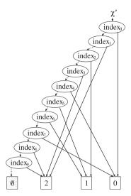
**Fig. 3** MTZDD for one-hot encoded function  $\chi'$  of h'.
