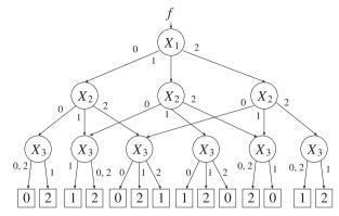
**Fig. 1** MDD for symmetric function f specified in Table 1.
