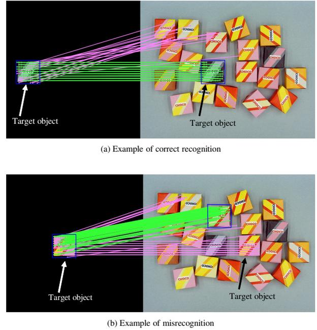
**Fig. 2** Successes and failures in recognition by related method (LoFTR) [25]. (a) is the result of correct recognition, (b) is the result of misrecognition. The proposed method makes these two cases recognizable.
