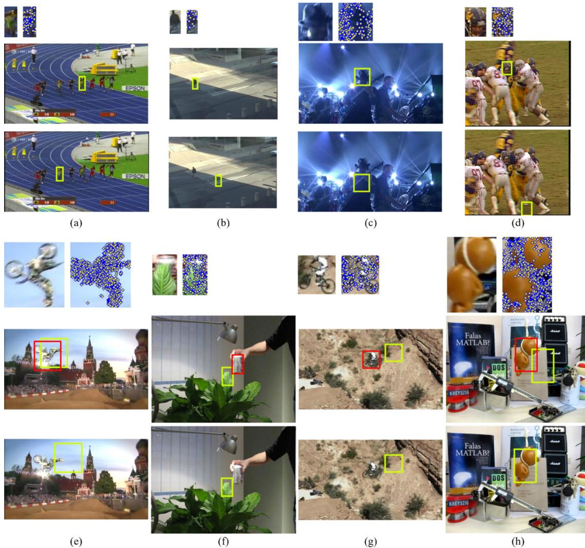
**Fig. 9** Recognition success and failure. Upper left: target image, Upper right: selected pixels. Middle: recognition result (Proposed method), Bottom: recognition result (BBS). The green line is the output result, and the red line is the GT.
