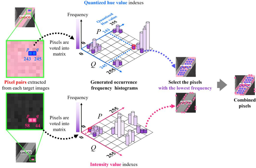
Fig. 4 Process of selecting effective pixels for matching in the target images.
